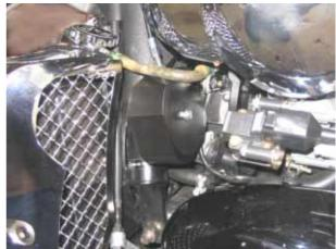
The **Control Switch** (6) is mounted to the left hand (clutch) master cylinder handlebar clamp and may be mounted below the left hand switch block (Lo mounting). There are two different designs of switch gear on Rockets. This photo shows the earlier design on the Classic. See over the page for the latest version of Rocket switch gear on the Touring. At this stage we believe that this later design is only fitted to the Touring.
