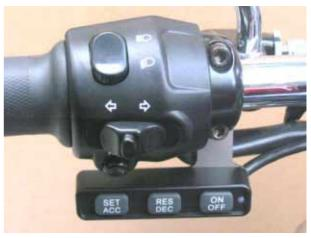
The mounting bracket may be reversed to mount the switch above the switch block if desired (Hi mounting). This applies to the early design switch gear only.
