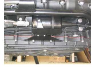
The CIU (4) is located on the left side of the bike, between the radiator and the throttle bodies, below the coolant header tank.
