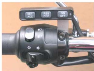
The two photos below are of the later design Triumph switch gear, in this case on a 2008 Touring. In this case the standard arrangement is to mount the switch above the bars (Hi mounting), using the same cruise control switch bracket as is used on the earlier models.
