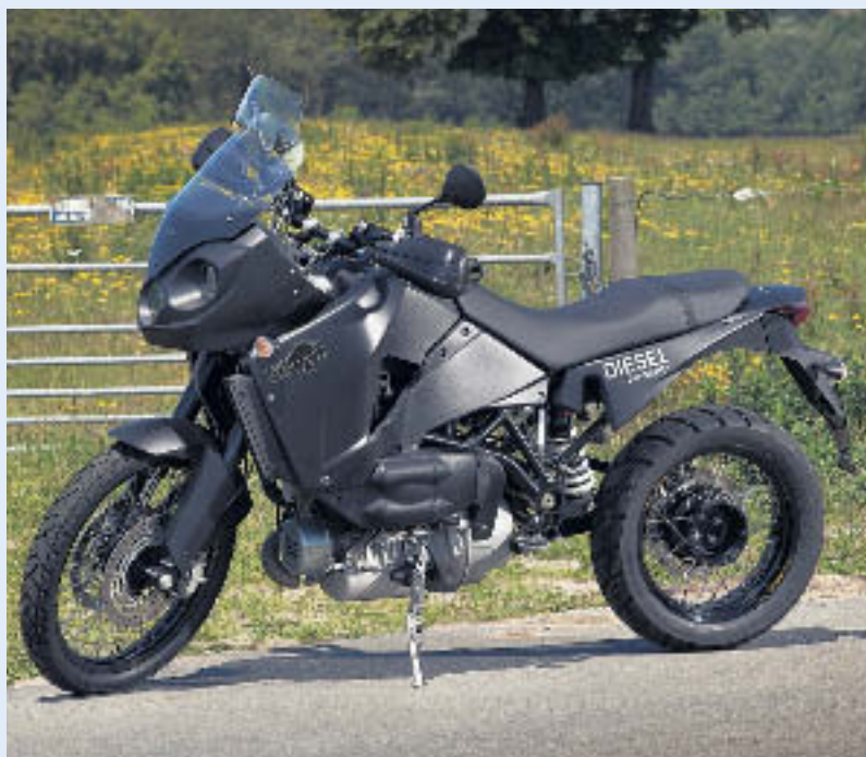
The Track uses same engine as diesel Tiger but has CVT and shaft drive
